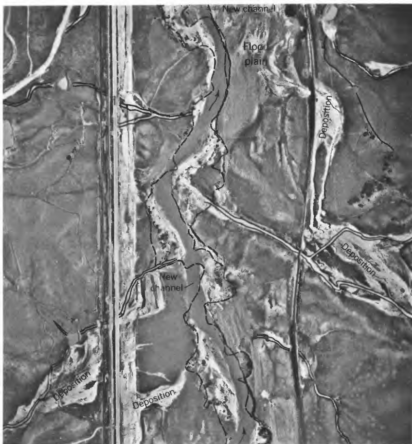
FIGURE 4.—Results of overland flow along East Plum Creek south of Castle Rock, Colo. Photograph by Colorado Army National Guard on June 18, 1965.
