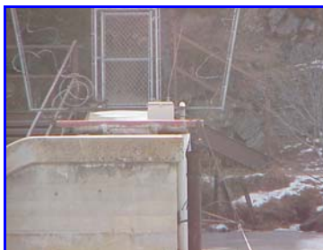
Figure 2.0: ALERT stream gage.
