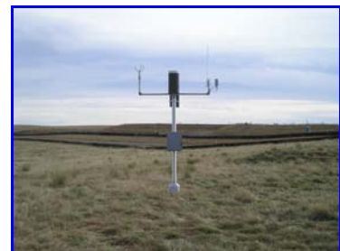
Figure 3.0: ALERT weather station.
